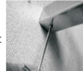
11. As shown in the picture, screw the grab screw (2) into the bracket hole (1) using the provided Allen tool; fix the bracket (1) onto the bush or short tube (3).
